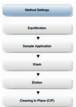
Fig 2.8. Typical phases of a chromatographic purification step.
